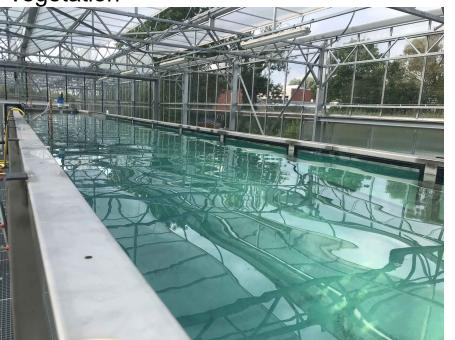
**FATI Platform ('Free-Air Temperature Increase')**: Infrared heater & rain out shelters + irrigation over 20 X 7m<sup>2</sup> of vegetation (grassland)
