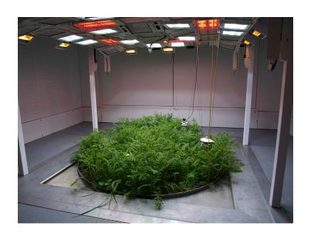
**TERRA-Ecotron**: 6 (8) closed units with artificial light (sun spectrum) in which climatic conditions are regulated over 2 m² of vegetation (lysimeters 1.5m depth). Configurated to study the impact of climatic events and evolution on agrosystem (plant-soil-water) interactions and yield
