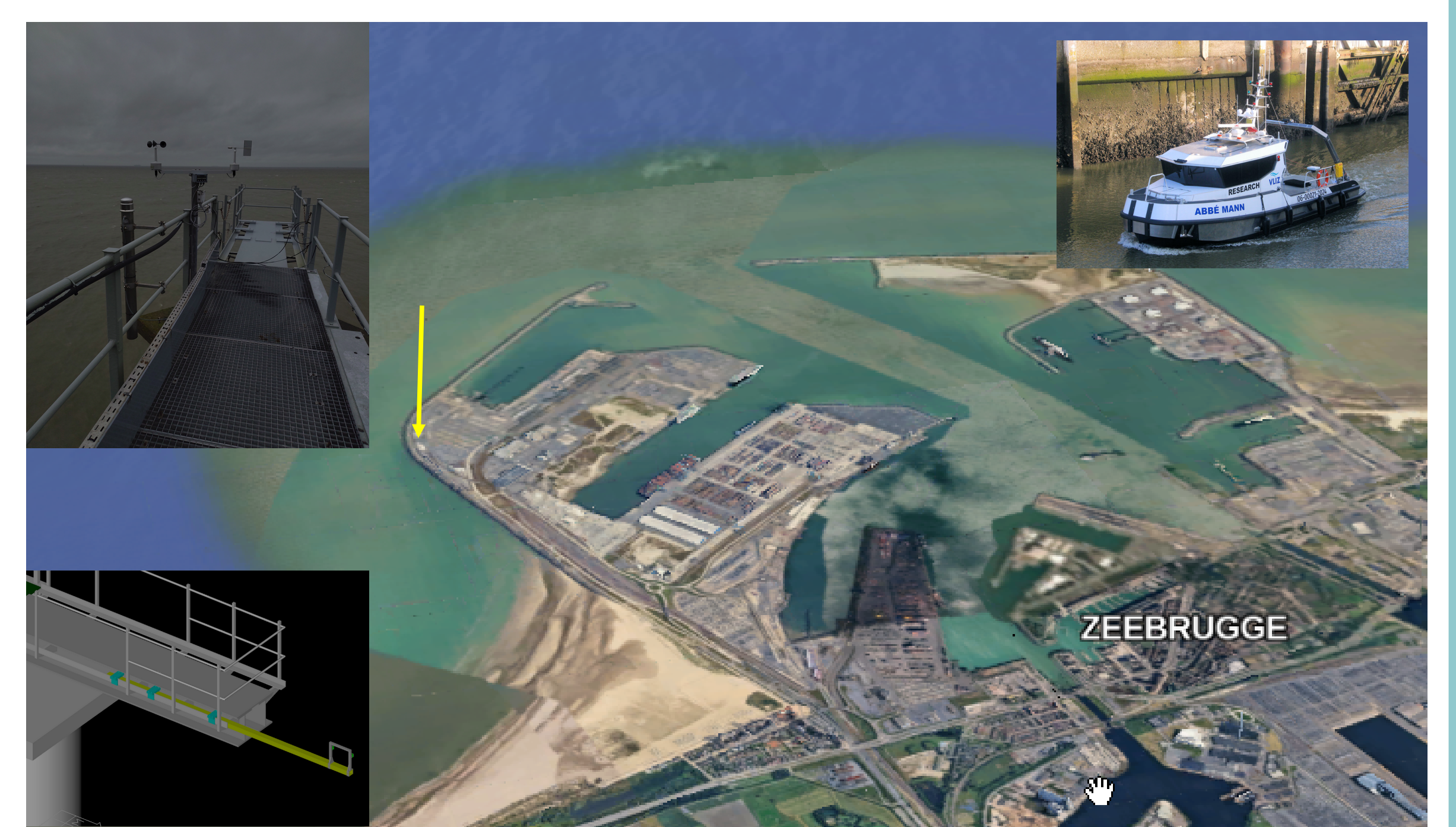
Fig. 3: Overview of the eddy covariance setup at the port of Zeebrugge. The setup will be installed on the western harbor head in collaboration with Flemish Hydrography, who manages the bridge structure (upper left inset). The sensor and gas intake will be installed 1-1.5 m outside of the bridge (lower left inset) at a height of ~15 m above the sea surface.
