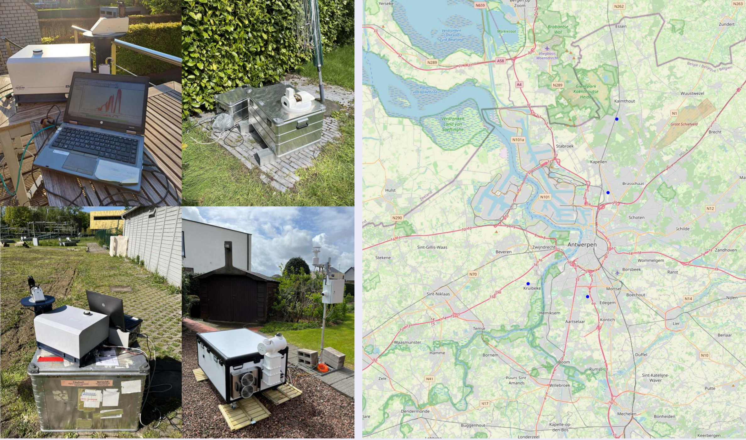
Figure: Left: KIT Bruker EM27/SUN in Ekeren, VU Amsterdam EM27/SUN enclosure in Heide, KIT EM27/SUN in Wilrijk, Bruker Invenio in a prototype BIRA-IASB instrument enclosure with solar tracker in Kruikebeke. Right: FTIR instrument locations around Antwerp during the FTIR campaign.
